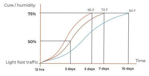
Curing time is affected by temperature and humidity.
